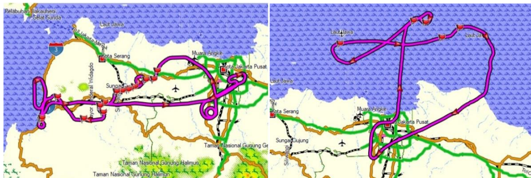
Figure 9: Weather modification technology to decrease rainfall intensities in Jakarta Greater Area. Purple line shows the track of cloud seeding that has been conducted on 3 January 2020. Source: BNPB.
